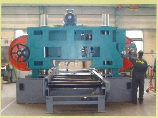
For the high speed resawing of large timber, the machines can also be supplied as a multi-head with a slatted bed feed system similar in construction to that of the MHS9 & MHS10.
