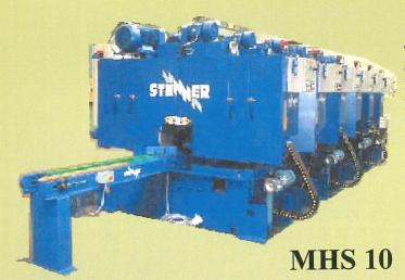
The sawing system has the capability and accuracy that only a Stenner can offer, combined with the robustness of construction and proven longevity of which the company is justifiably proud. It includes pressure sawguides, pneumatic saw straining and ducted sawdust extraction as standard.
