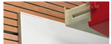
Laser-assisted indication of the horizontal cut (standard)
