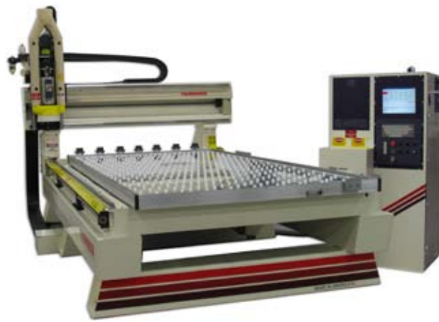
Thermwood fixed table machines have separate servo drives for each side of the gantry to prevent skewing and provide independent compensation for each lead screw, assuring squareness and accuracy.
