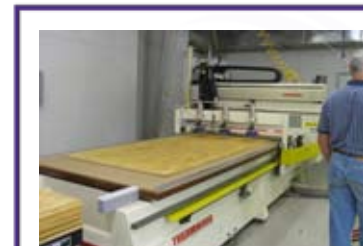
Using Automatic Load and Unload a single operator can run more than one upholstered frame system.
