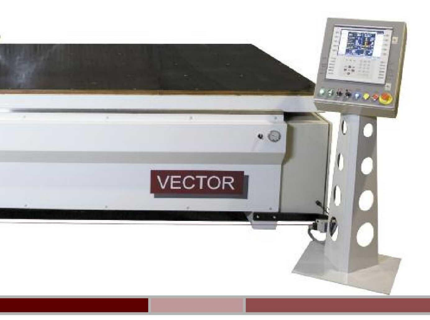
The **VECTOR** *Revolution 180* is the first Contour Edgebander to adopt 'Simultaneous Processing' where all functions are performed simultaneously rather than sequentially.
