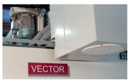
The joint of the edge where a complete 360 degree edging is required is controlled by a sensor arm. The speed of approach is automatically reduced at a precise distance from the joint and a sensor accurately detects the beginning of the edge which remained untrimmed at the cycle start. The trim cutter then cuts the edge with a bevel, the edge is applied and the top/bottom trimmed leaving a joint of the highest quality.
