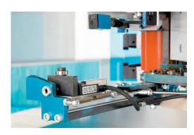
Where square cornered panels are to be processed the VECTOR Revolution 180 uses special EndPODS. These pods incorporate starting and finishing plates which simulate an extension of the workpiece. The advantage of this system is that it gives a reference for the panel placement and equally importantly provides a straight edge to lay down the initial banding.
