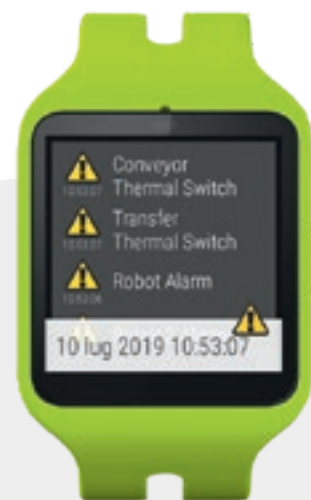
NOTIFICATIONS List of alarms or maintenance requests. Every time the machine signals that there is a problem, or when there is a maintenance request, the Viet Watch vibrates and a danger icon is displayed on the screen.
