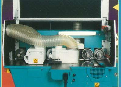
Both the near side and top head chipbreakers are of the Wadkin radial type ensuring maximum safety even with larger variations in timber sizes. The radial chipbreaker allows the ultimate in control of thin or narrow sections and eliminates unevenness on the end of the timber.
