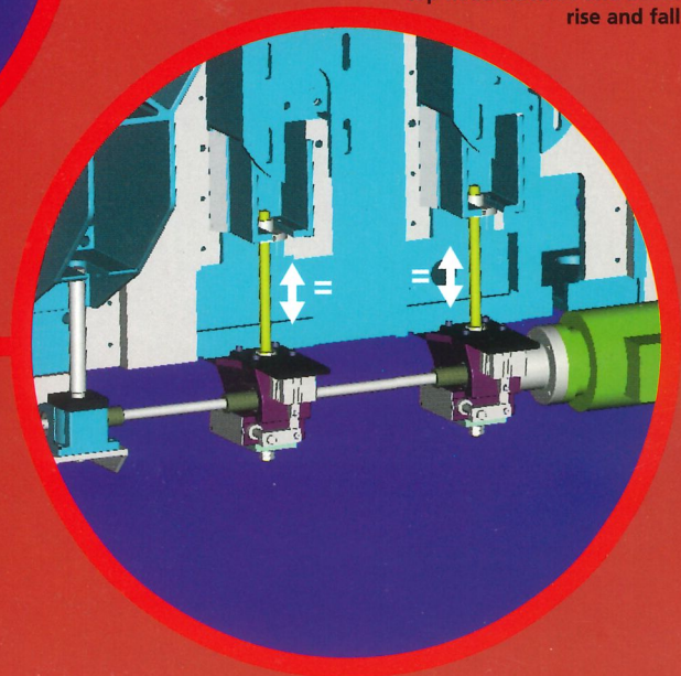
Synchronised operation of top head clutches and beam rise and fall
