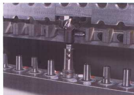
Changeable support segments for drilling outside of the panel field
