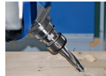
Drilling and routing in different angles
