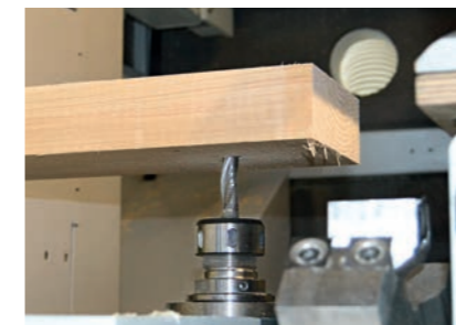
Milling a tenon hole with the underfloor unit
