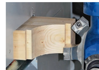
Machining the rafter head
