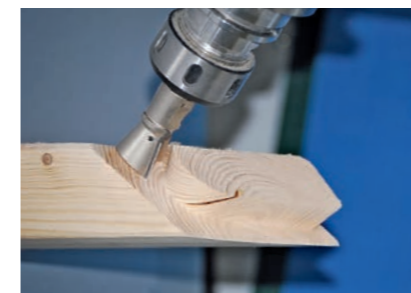
Dovetail at the jack rafter
