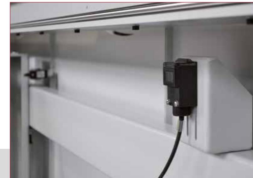
Laser photocell for required panels counting on each specific manufacturing process.
