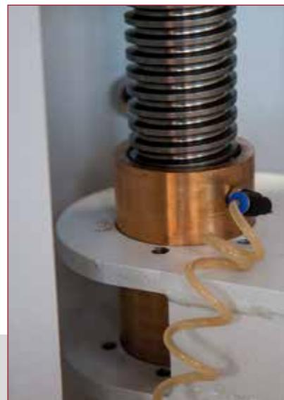
Motorized lifting with 4 x 50 mm diameter screws and self-lubricating bronze screw nuts.
