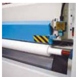
Panel thickness Control barrier with emergency stop.
