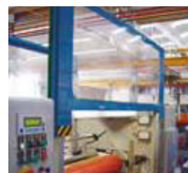
Upper protection with total visual access and prepared for gas extraction
