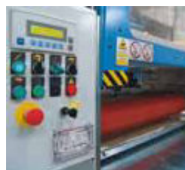
Glue grammage adjustment by speed variation.
