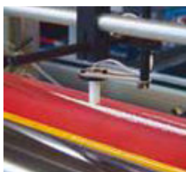
Level detectors for the glue supply control.
