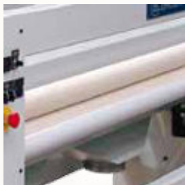
Flat top and bottom pressure rollers.
