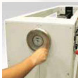
Raising through manual spindle with analog indicator.
