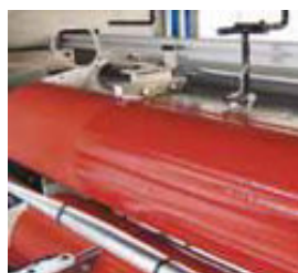
Applicator roller coated with silicone rubber.
