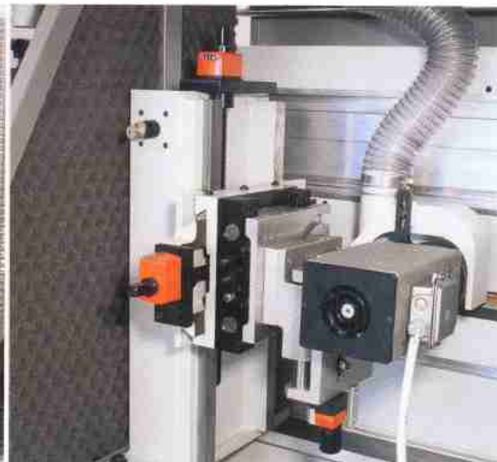
Universal milling unit with pneumatic jump, 0-90° rotatable.
