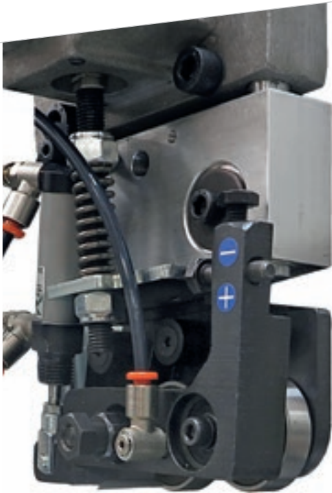
Buffing unit to clean and polish the edge and the panel.
