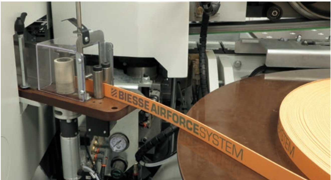
Single-roll automatic loader , enables rapid change of the edgebanding strip with no need to open the cabins. Optic sensor for detecting the correct positioning of the edgebanding strip (opt.).
