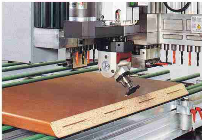
Cutting operations with tilted saw. Nuten mit beliebigem Winkel
