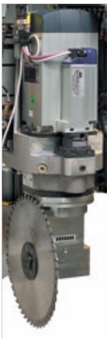
The multi-function unit, which can be continuously positioned over 360° by NC, can house aggregates used to carry out specific machining operations (pocketing for locks, hinge housings, deep horizontal bores, edge trimming, etc.).
