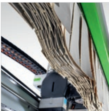
Side curtain guards to protect the working unit, which are movable to enable the machine to work at maximum speed in total safety.
