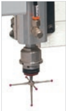
The cross-head thickness tracer enables operators to measure panel dimensions with absolute precision.
