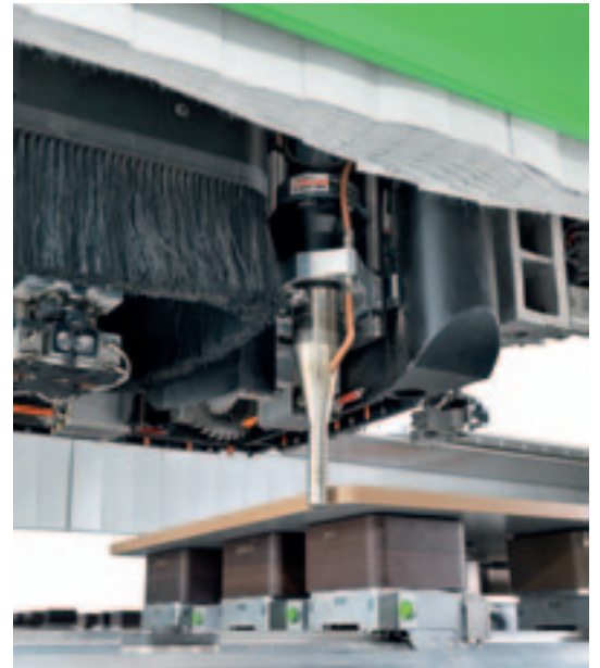
Blower unit with hot or cold air.
