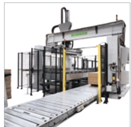
BIESSE WINNER UNLOADING AND STACKER SYSTEM Bridge stacker with pincer frame to handle packs of panels.
