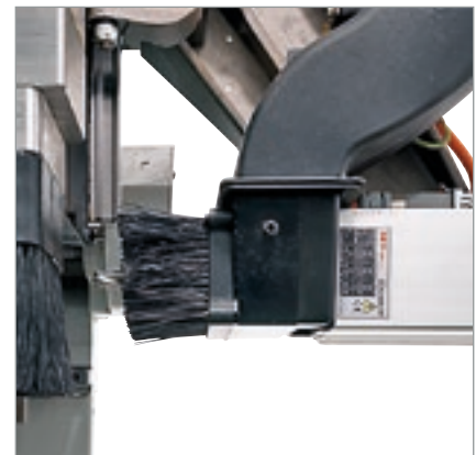
Fixed horizontal motor with one outlet for lock routing and horizontal machining operations.
