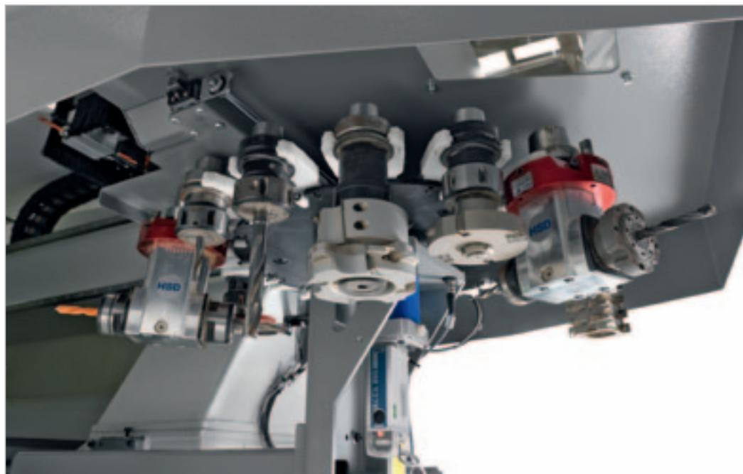
Revolving tool changer with 16 places. Installed on the X carriage, it allows to have tools and aggregates always available therefore reducing the tool change time.
