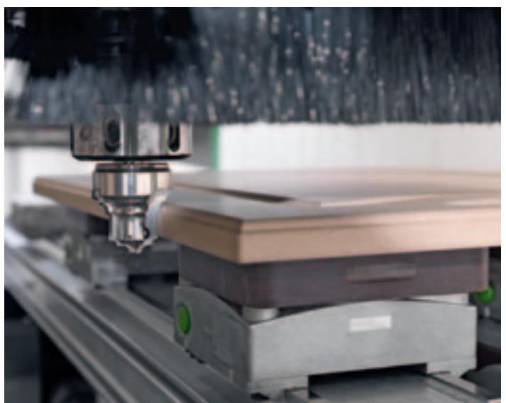
Machining of core panel and element door.
