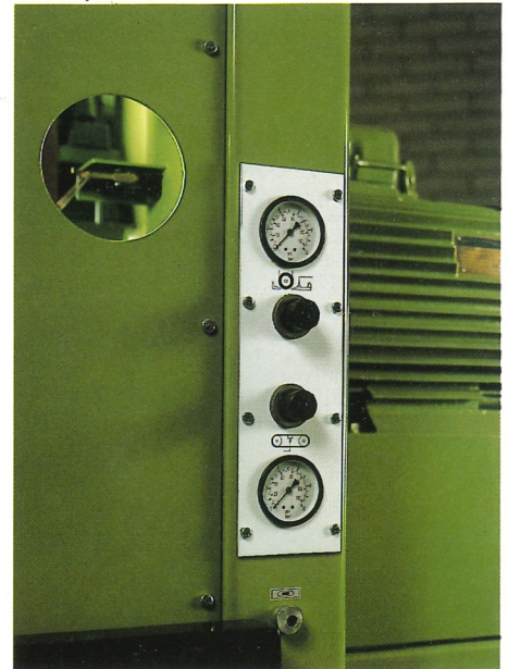
Control panel for table and infeed pressure bar adjustment.
