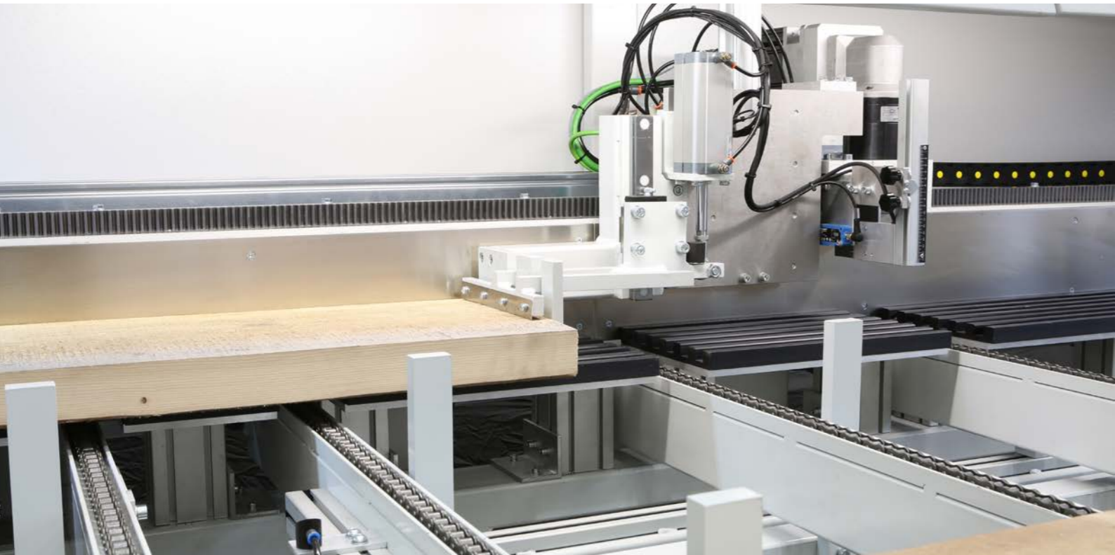
^ Pusher-carriage with top-bottom pneumatic clamp
