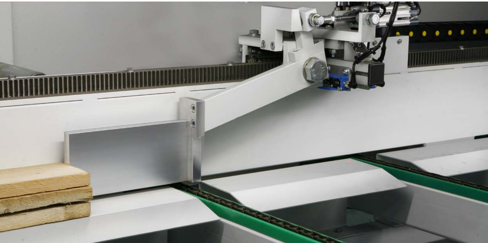
^ Pusher-carriage with top-bottom pneumatic clamp
