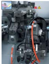
Trimming unit Multifunctional trimming unit with DFC (Dust Flow Control) tooling technology for optimal extraction. Optional pneumatic or servo axis adjustment available.
