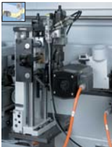
Universal trimming unit Universal unit with high capacity for grooving and profiling work. Flexible by unlimited setting options.
