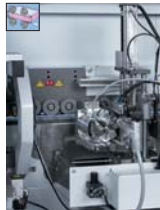
Multifunctional trimming unit (optional) Trimming of the edge overhang on top and bottom side as well as contour trimming on the front and rear edges. Equipped with an automatic adjustment to switch between thick and thin edges. Workpiece thickness up to 60mm.
