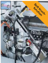
End trimming unit Perfect cutting by the end trimming unit using rigid high-precision linear guides and the workpiece gap optimization package to achieve higher output in the same processing time. Soft-touch for optimal end trimming results even at high speeds.
