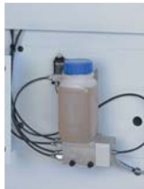
Central lubrication unit Fully automatic lubrication of the feed track guidance system to guarantee precision and a long-life time of the conveyor chain.
