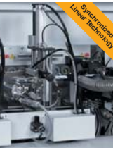
Multifunctional trimming unit (optional) Trimming of the edge overhang on top and bottom side as well as contour trimming on the front and rear edges. Equipped with an automatic adjustment to switch between thick and thin edges. Workpiece thickness up to 60mm.
