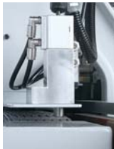
Infeed stop For minimum workpiece spacing and safe operation.
