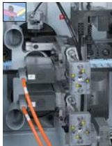
Rough trimming unit For rough trimming of all common edgebanding materials.
