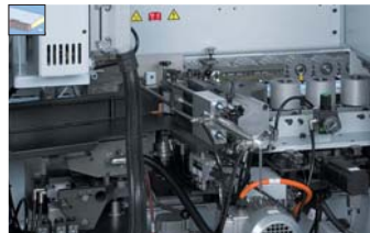
Magazine + pre-melter (optional) Coil and automatic strip magazine with optical monitoring for reliable material supply, high availability and perfect glue quality via the Quickmelt gluing unit.
