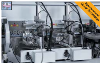
Multifunctional trimming unit (optional) Trimming of the edge overhang on top and bottom side as well as contour trimming on the front and rear edges. Equipped with automatic adjustment to switch between thick and thin edges. Workpiece thickness up to 60mm.
