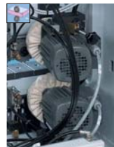
Buffing unit Buffing unit to polish edges and maintain their natural color.
