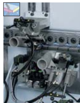
Profile scraping unit Unit to smooth radii or chamfers, equipped with quick change heads for fast profile change.
