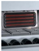
Radiant heater Strong adhesion through optimal pre heating of the workpiece.
