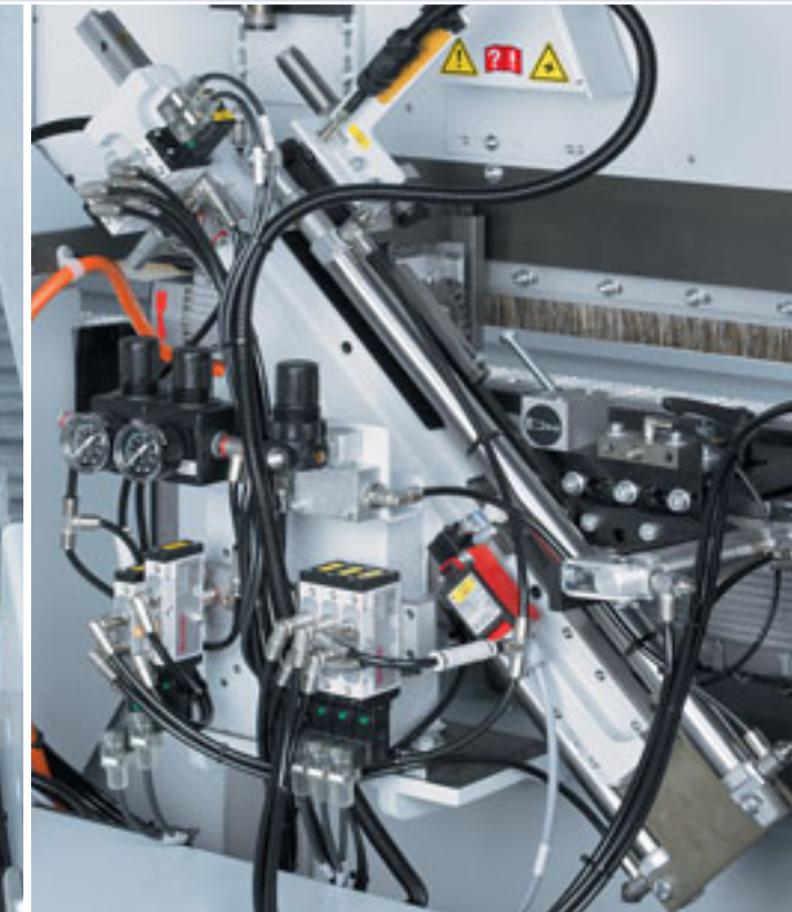
End trimming unit Perfect cutting by the end trimming unit using rigid high-precision linear guides and the workpiece gap optimization (optional) package to achieve higher output in the same processing time. Soft-touch for optimal end trimming results even at high speeds.
