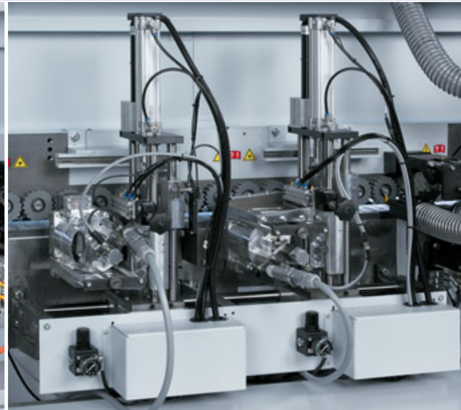
Multifunctional trimming unit (optional) MF 50 Trimming of the edge overhang on top and bottom side as well as contour trimming on the front and rear edges. Equipped with an automatic adjustment to switch between thick and thin edges. Workpiece thickness up to 60 mm.
