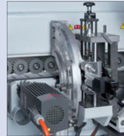
Nesting package (optional) Includes a multi-roller tracing device for the trimming and scraping units to compensate for hinge holes.
