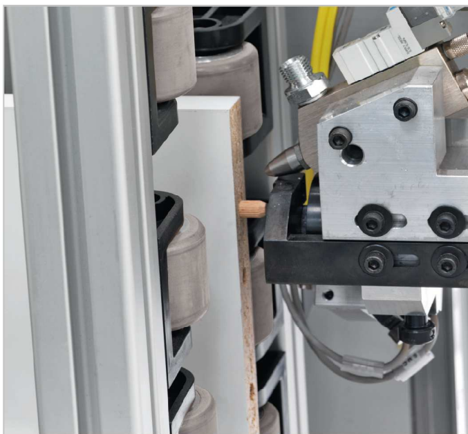
Glue & dowel inserting unit placed on the rear side of the column mounted on controlled axis Y.
