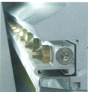
Oscillating air-jet belt blower, activated by the workpiece
