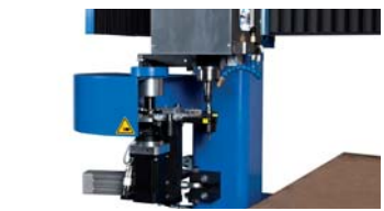
Tellerwechsler 8-fach, optional 8-time Disk type tool changer, optionally
