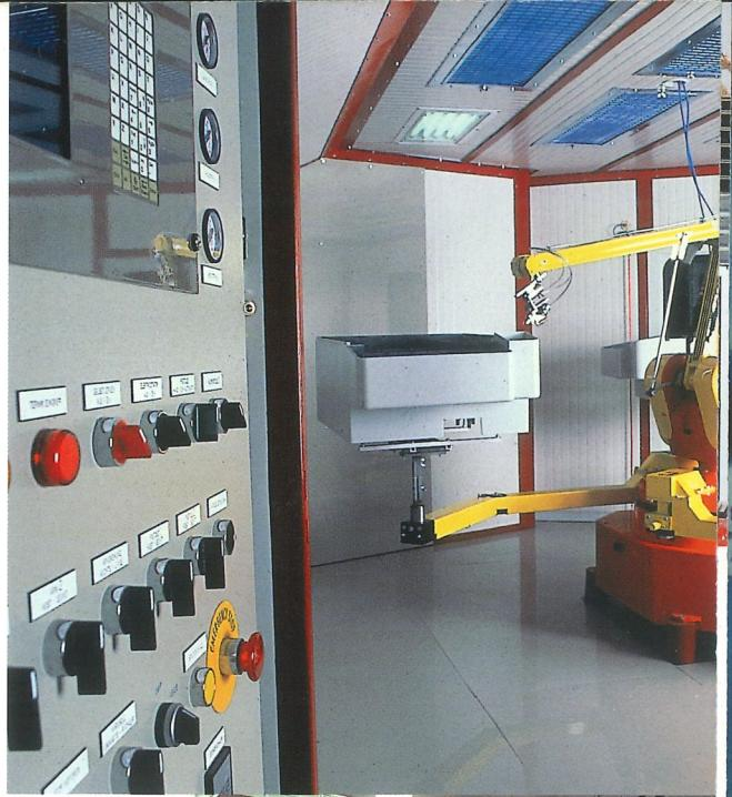
*Version with carousel* with two-or-more arms; the pieces to be painted are loaded at the back of the Robot in a safe area; the carousel provides for the positioning of the piece at the frontal side for the working, and recarries it at the back for the unloading. Each arm is equipped with supporting system and rotation of the piece controlled during the programming phase.
