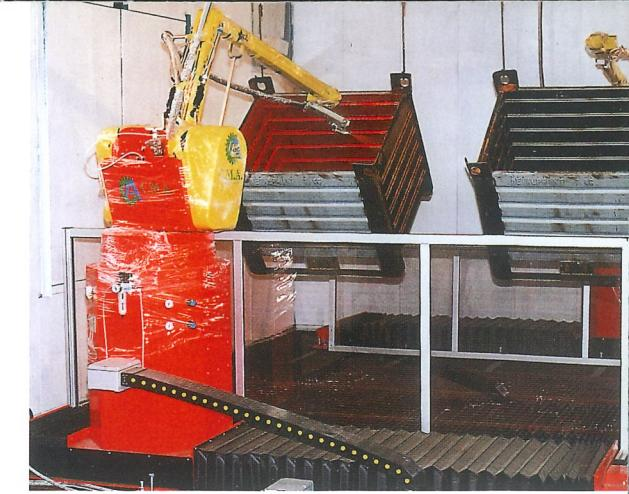
ST version mounted on electrically operated cart, it is utilized for the painting of particulars of considerable dimensions. The Robot synchronizes itself with the speed of the conveyor, effects the cycle moving, and goes back to the waiting position for the following piece. Programming can take place both with the piece firm, and moving. The speed of the cart perfectly adapts itself to that of the conveyor.
