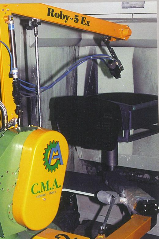
**Version with carousel** with two-or-more arms; the pieces to be painted are loaded at the back of the Robot in a safe area; the carousel provides for the positioning of the piece at the frontal side for the working, and recarries it at the back for the unloading. Each arm is equipped with supporting system and rotation of the piece controlled during the programming phase. Robot arms shrink to reduce the space taken up by the carousel rotation.
