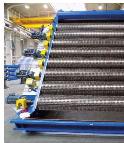
Outfeed rollers gently discharge the fibers to protect their geometry. Design ensures an uniform material discharge
