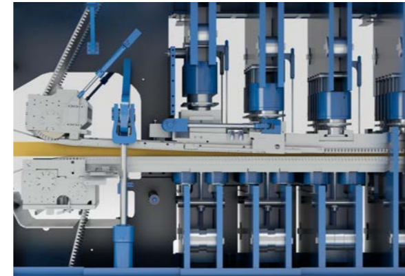
01 Double-hinge infeed system for fast pressure and temperature buildup
