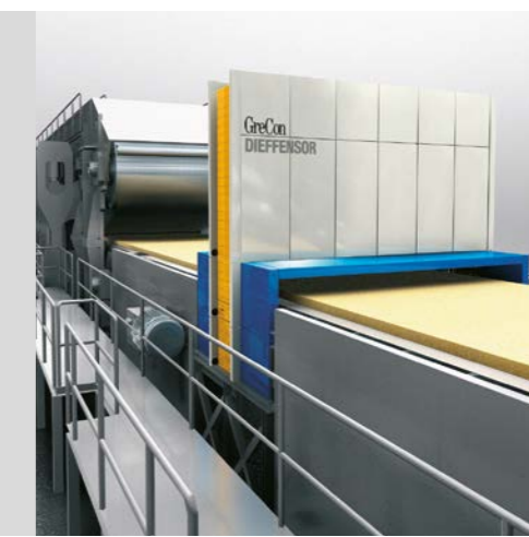
Dieffensor senses area densities crosswise and lengthwise with high resolution
