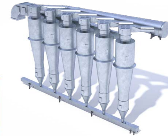
08 Cyclone battery: Optimized by using the fluid dynamics (CFD) analysis to improve separation efficiency and pressure loss.
