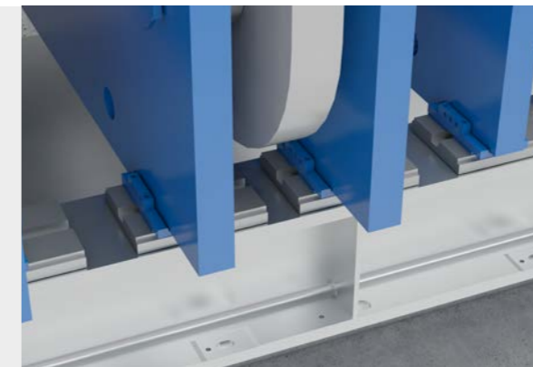
07 Thermal expansion compensation—unrestricted temperature changes during production
