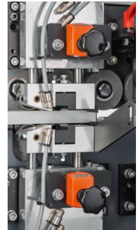
Surface scraper with dual-tracing (optional)
