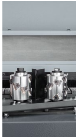
Diamond-tipped pre-milling aggregate
