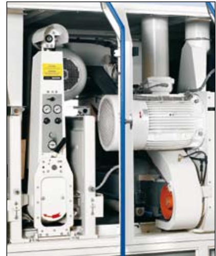
Steel roller with precision bearings followed by a cross sanding unit
