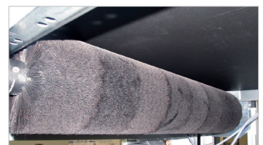
Belt cleaning equipment
