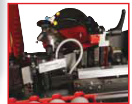
Stanz- und Leimaggregat punching and glueing device
