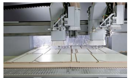
Synchronous processing during the nesting of carcase furniture components
