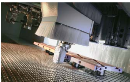
Staircase stringer processing on Flex-System
