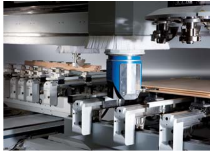
Simultaneous processing of a door frame and door leaf
