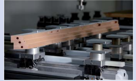
The pneumatic clamps are traversed after longitudinal profiling of parts such as window staves in the Y direction for 5-sided processing
