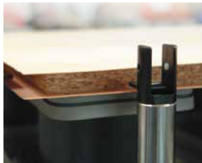
Stops for coating ply overhang (optional) Ensures easy positioning in the case of coating ply overhang (e.g. veneer)
