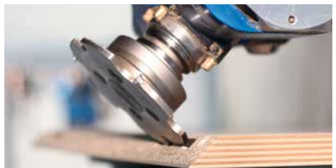
Cutting recesses for connecting fittings
