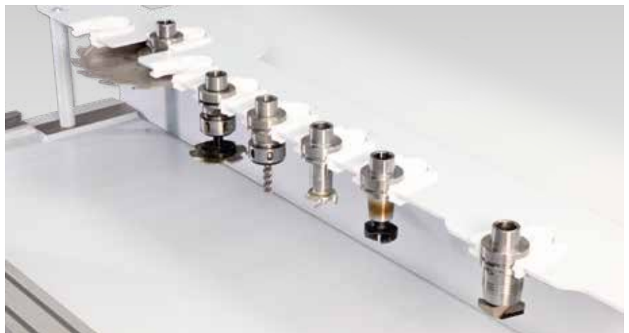
7-slot linear tool changer [5-axis version] – additional tool changing magazine with 7 slots and integrated tool pick-up station, laterally installed. One slot is prepared to accommodate a saw with a diameter of 350 mm.
