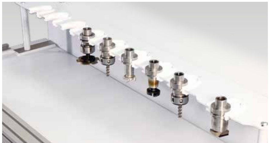
8-slot linear tool changer [3-/4-axis version] – additional tool change magazine with 8 slots and integrated tool pick-up station, laterally installed.
