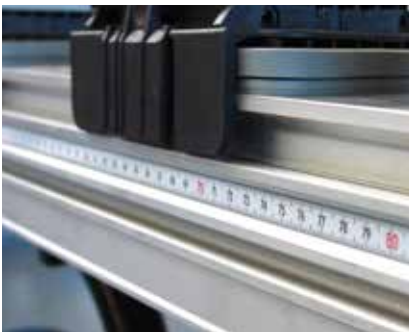
Measuring tape For positioning of suction cups
