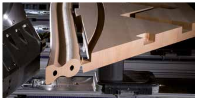
Holes for piling at narrow angles
