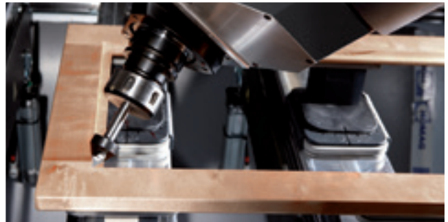
Square corner routing for a glass rebate
