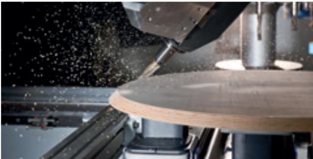
Chamfer trimming on a table top
