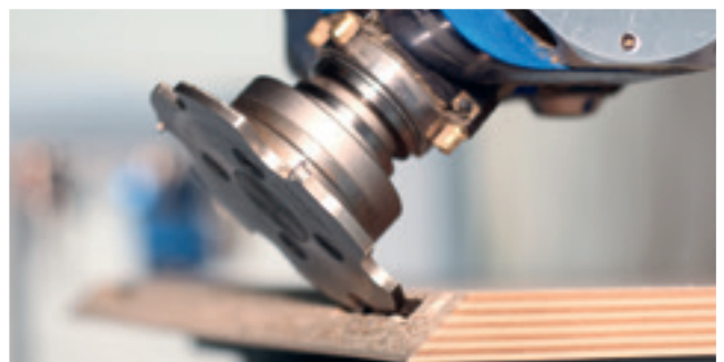
Cutting recesses for connecting fittings
