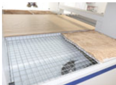
Large filters are easily accessible and replaceable for cleaning and maintenance.
