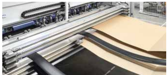
The continuous cardboard changer is an automatic changing system for continuous track widths with up to six slots.
