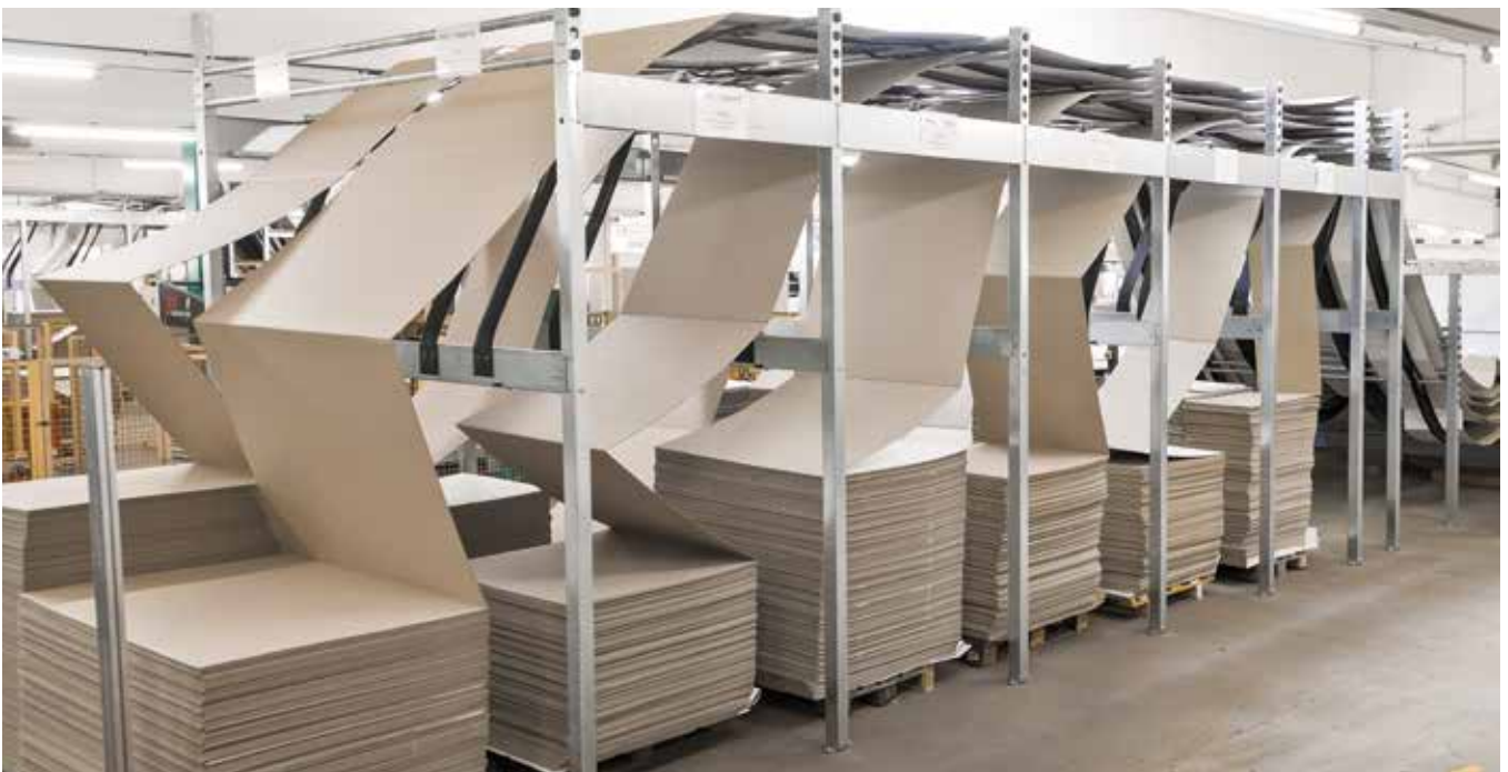
In side-by-side operating mode, a further track width is added to the cardboard box feed slot so that with a six-slot change system, up to 12 track widths are possible, each with individual access.
