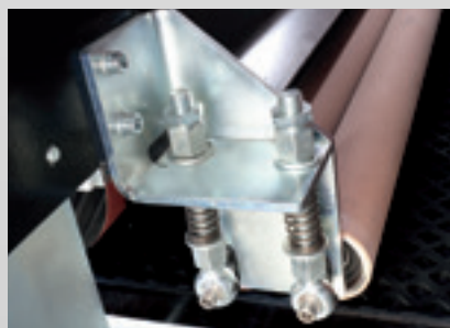
Solid guidance by rubber-covered pressure rollers Spring-loaded pressure rollers with solid guidance. The pressure elements are situated with minimum distance to the intervention area. An additional pressure roller is in front of and behind the workpiece detection.
