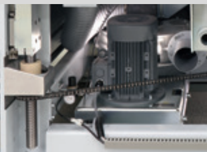
Workpiece thickness setting by four threaded spindles adjusting the upper machine frame.
