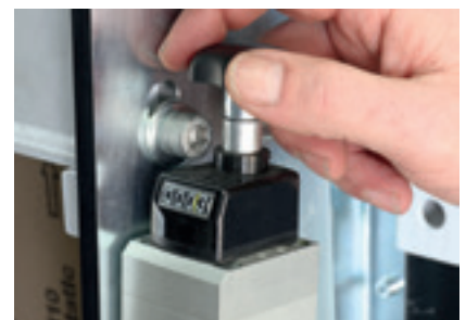
Standard Contact roller with manual grain size offset
