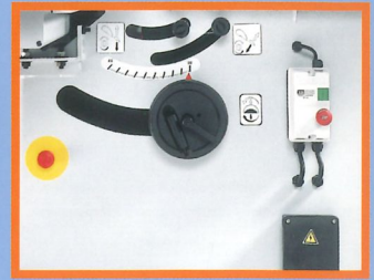
User-friendly design for scoring adjustment, magnetic switch.
