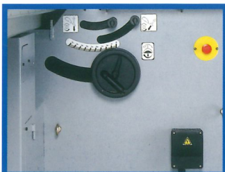
User-friendly design for scoring adjustment, magnetic switch.
