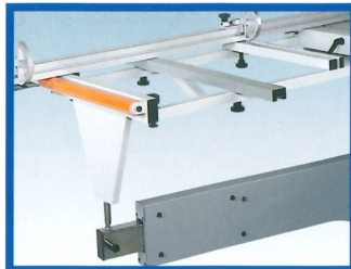
Strong outtrigger and large support roller for loading panel smoothly.
