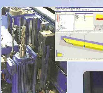
The optional vertical mill unit, can be fit with a variety of different mills and can be used to produce dados, vent holes and corbels, etc..
