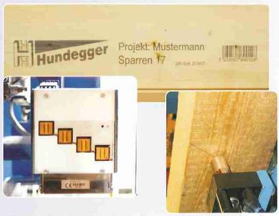
The optional printer unit can be used to create layout lines and can be used to label parts with text. Text heights range from 12,7 to 50,8 mm on one or up to four lines.
