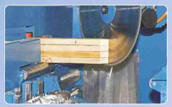
Any type of part can be efficiently processed from any size and length of lumber including EWP. By using Hundegger'soptimization program, same angle parts can be groupedtogether for faster production and less waste.
