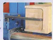
The horizontal drill can perform through or blind drillings. A rafter drilling is shown here
