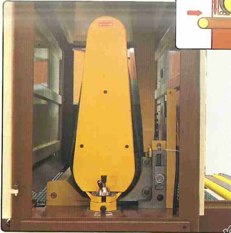
SRN Gauging-Sanding machine with one operative unit
