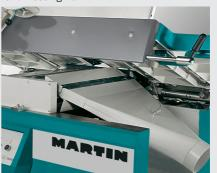
Idle rollers in the thicknessing table help to support and feed large cross-sections of wet
