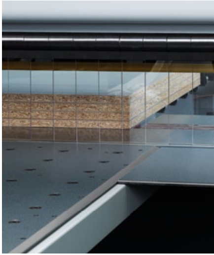
Sturdy steel pressure beam with variable opening height.
