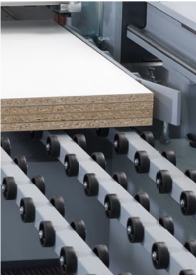
Roller tracks on the rear support table for smooth panel handling to the cutting line.
