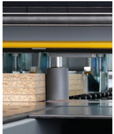
Double performance pressure unit – uncompromisingly precise positioning against the mitre fence.
