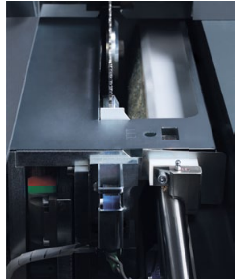
Sophisticated saw carriage guides that minimize wear and tear ensure the perfect 90° cut every time, even after years of continuous industrial use.
