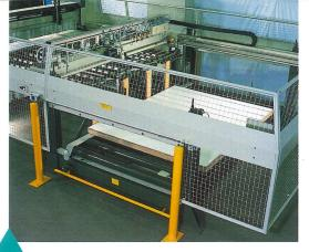
The lifting table is fitted with driven heavy-duty roller conveyors. Panel stacks can be positioned on the lifting table from the left, right or behind. To turn the panel pack automatically the machine can be equipped with a turning table in the rear machine bed.
