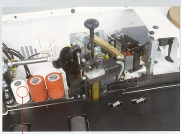
Three rollers pressing the edge band onto the panel. One nylon roller and two rubber-coated rollers. One of the rollers pivots.
