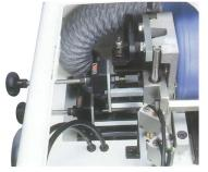
Trimmer unit adjustment is easy thanks to the precision numeric indicators. These give precise position readings to tenths of a millimetre. They ensure an easy, rapid return to previous settings.
