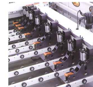
高性能气动式送料夹钳 Pneumatic clamping for best feeding performance
